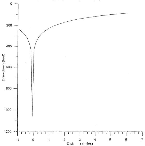
Regional drawdown in the Cambrian-Ordovician aquifer produced by 1 well pumping 7500 GPM. (T= 20,000 gpd/ft2, S = 0.0004, time = 1 year)
